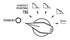
There is a manual switch for selecting the various welding processes on the welding control panel. There are 5 processes to choose from:
